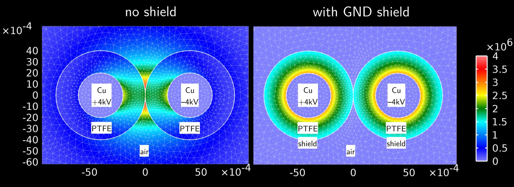
Electric field FEM of two electrical cables in air.
